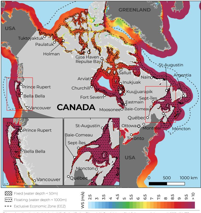
This map shows the estimated technical potential for fixed and floating offshore wind in Canada in terms of installed power capacity in megawatts (MW) within 200 kilometers of the shoreline. It is provided by the Global Wind Energy Council (GWEC) with funding from the Ocean Renewable Energy Action Coalition (OREAC), to support the UN High Level Panel for a Sustainable Ocean Economy (Ocean Panel). For more information visit: https://gwec.net/oreac/.
