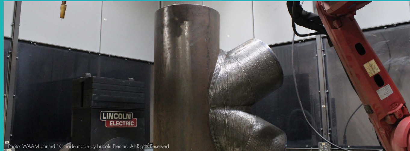
Photo: WAAM printed "K" node made by Lincoln Electric, All Rights Reserved
